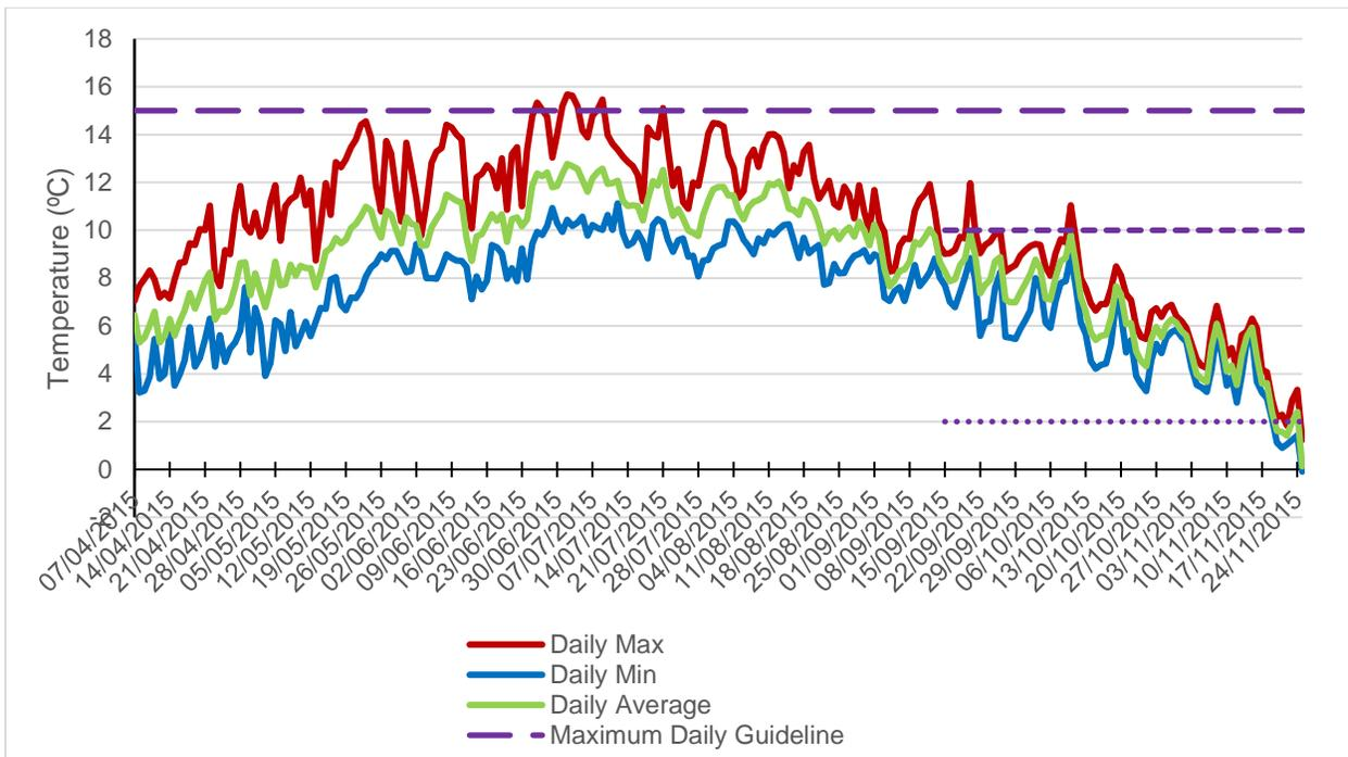
**Figure 1. Stream water temperatures in Windermere Creek (site NAWIN03) from April 7 to November 25, 2015. The long dashed purple line indicates the BC MOE guideline for aquatic life for streams with Bull Trout present. The short dashes indicate maximum daily temperature during spawning, and the dotted line indicates minimum daily water temperature during spawning and incubation.**
