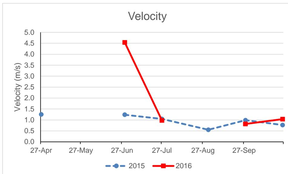
**Figure 2. Water velocity at McDonald Creek (NEMCD01) in 2015 and 2016. No measurements were taken in May for both years due to safety concerns during high flows, and in August 2016 due to an equipment issue.**
