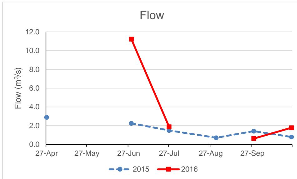
**Figure 3. Water flow at McDonald Creek (NEMCD01) in 2015 and 2016. No measurements were taken in May for both years due to safety concerns during high flows and in August 2016 due to an equipment issue.**
